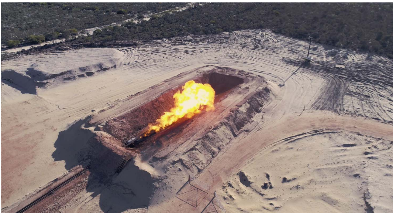
Above: Waitsia-3 flow test produced a peak rate of 50 MMscf/d and an average rate of 49.5 MMscf/d, October 2017.
