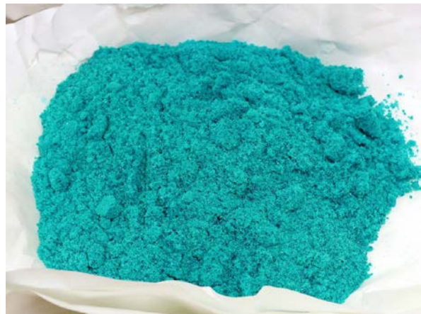
Approximately 1.6 kg of nickel sulphate hexahydrate crystals were produced in the recent test campaign. (Photography by: Karel Osten, Wood Plc)
