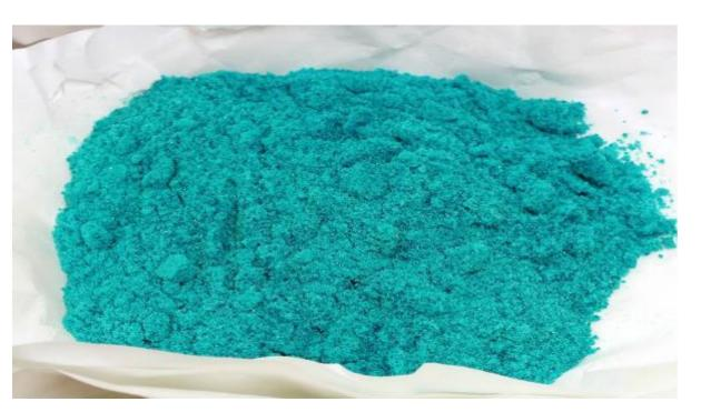
Photographs to the LHS are of the 1.6kg of nickel sulphate hexahydrate crystals produced in the metallurgical testwork. Photography by Karel Osten, Wood Plc
