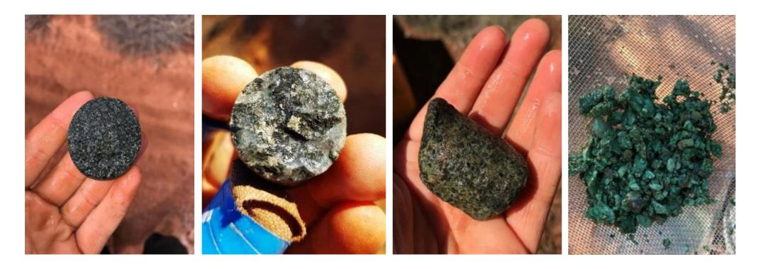
2018 examples of (from left) mafic granulite, Cu-Ni sulphides in gabbro, olivine websterite containing elevated Cr and fuchsite containing >1% Cr in some of the AC drill holes.
